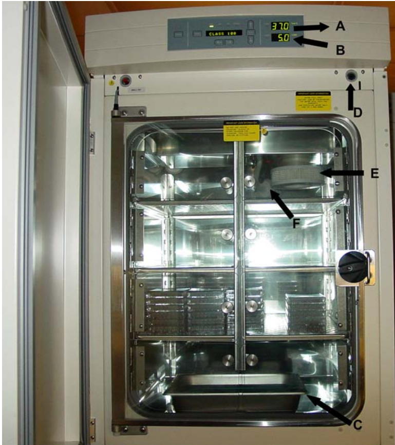
Fig. 2. CO 2 water-jacketed oxygen and eight CO 2 -regulated incubator (Model 3110 from ThermoForma, Marietta, OH), which has eight smaller inner doors separating the incubator into eight chambers. (A) Temperature display; (B) % O 2 display; (C) humidity pan; (D) water jacket fill port; (E) HEPA filter; (F) O 2 sensor.
