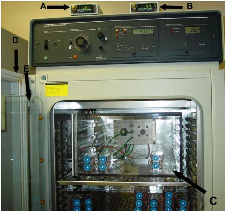
Fig. 3. PROOX model 110 (Reming, Redfield, NY). (A) CO<sub>2</sub> controller; (B) O<sub>2</sub> controller; (C) hypoxia chamber inside a host incubator; (D) outer door; (E) inner door.
