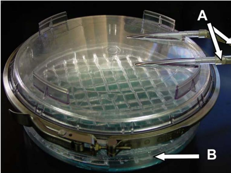
Fig. 4. O<sub>2</sub>-controlled chamber (Billups-Rothenberg, Del Mar, CA). The sealed, humidified, modular incubation chamber is flushed with a gas mixture and sealed to obtain hypoxic conditions. (A) Inlet and outlet tubes; (B) sterile, distilled water.
