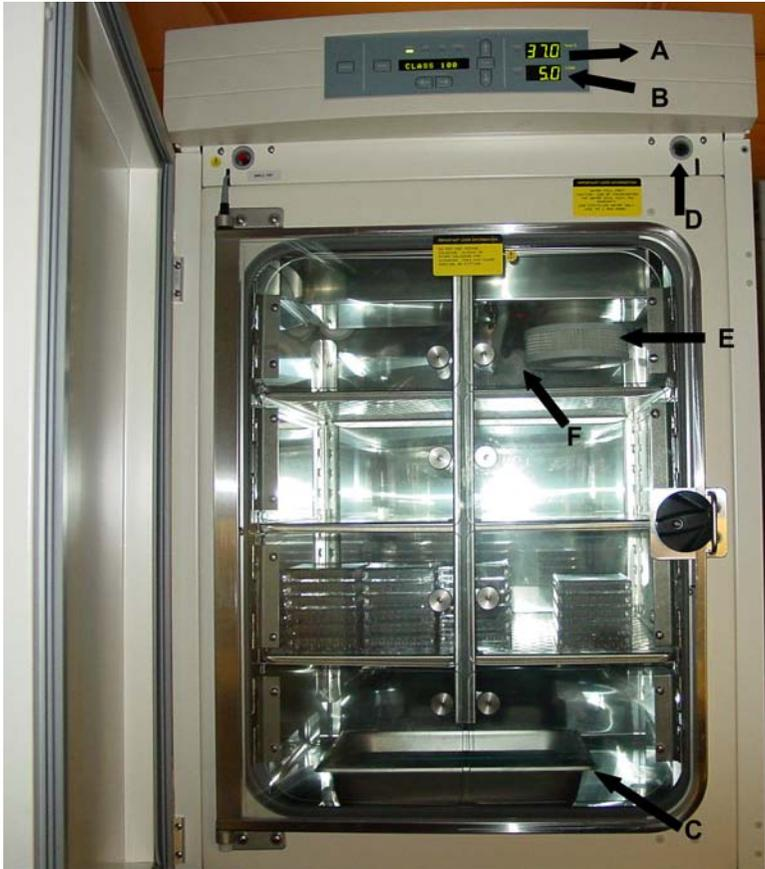
Fig. 2. CO<sub>2</sub> water-jacketed oxygen and eight CO<sub>2</sub>-regulated incubator (Model 3110 from ThermoForma, Marietta, OH), which has eight smaller inner doors separating the incubator into eight chambers. (A) Temperature display; (B) % O<sub>2</sub> display; (C) humidity pan; (D) water jacket fill port; (E) HEPA filter; (F) O<sub>2</sub> sensor.
