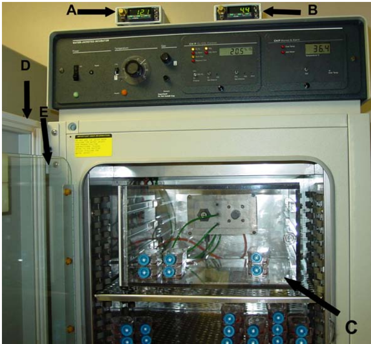
Fig. 3. PROOX model 110 (Reming, Redfield, NY). (A) CO 2 controller; (B) O 2 controller; (C) hypoxia chamber inside a host incubator; (D) outer door; (E) inner door.
